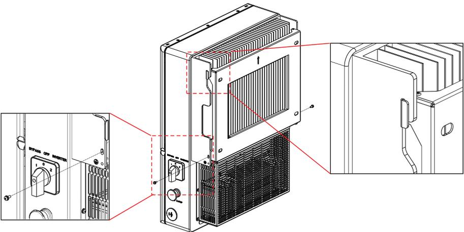
Figure 5.11 Inverter on mounting bracket and set screws
