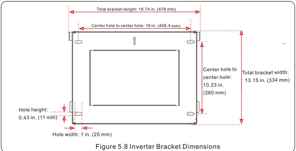
Figure 5.8 Inverter Bracket Dimensions
