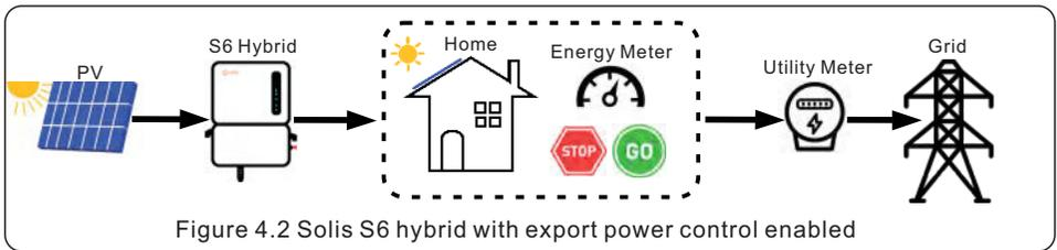
Figure 4.2 Solis S6 hybrid with export power control enabled
