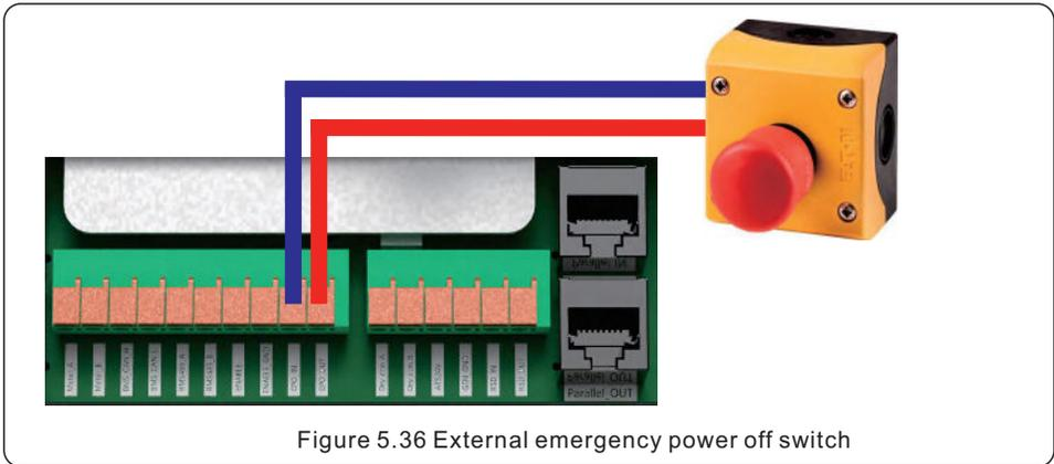
Figure 5.36 External emergency power off switch
