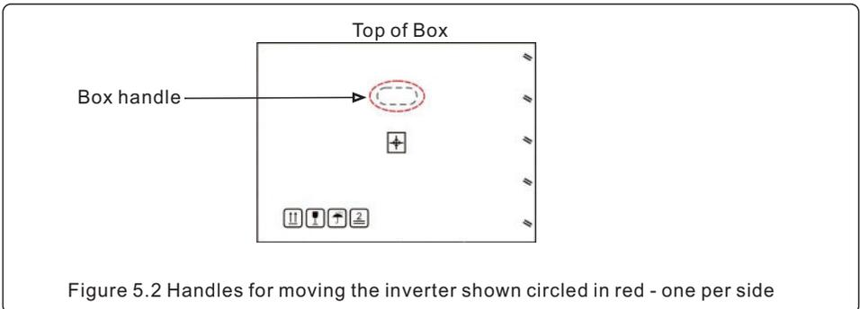
Figure 5.2 Handles for moving the inverter shown circled in red - one per side
