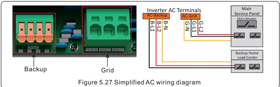
Figure 5.27 Simplified AC wiring diagram
