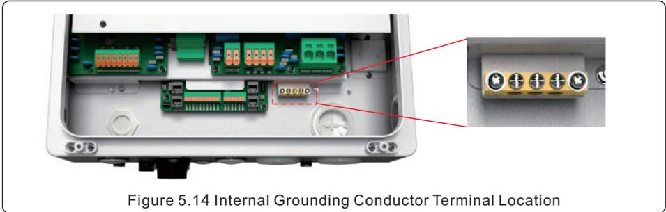
Figure 5.14 Internal Grounding Conductor Terminal Location
