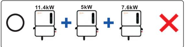
3. Paralleled inverters must have the same capacity (kWh), brand, and model of battery connected.
