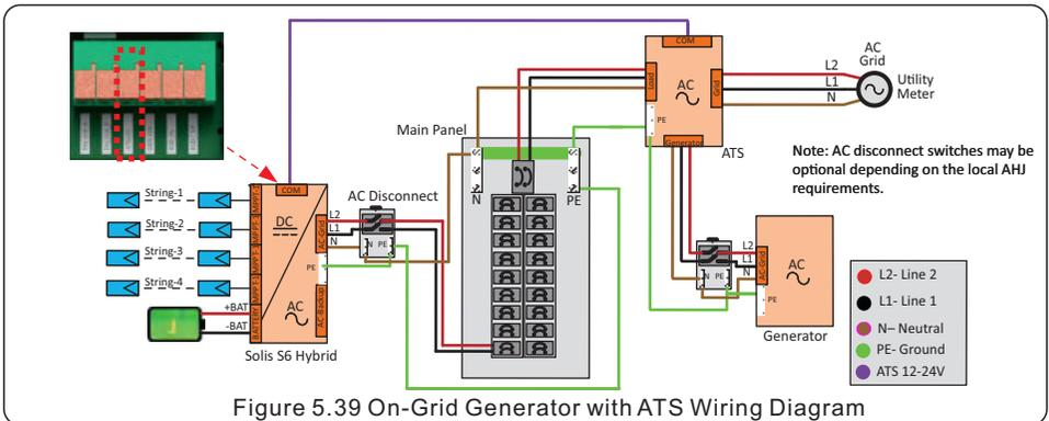
Figure 5.39 On-Grid Generator with ATS Wiring Diagram
