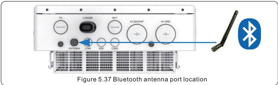
Figure 5.37 Bluetooth antenna port location
