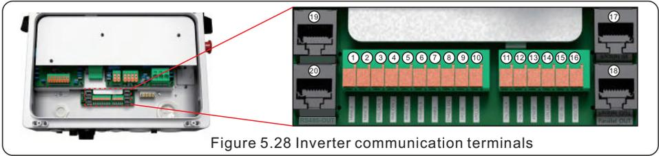
Figure 5.28 Inverter communication terminals
