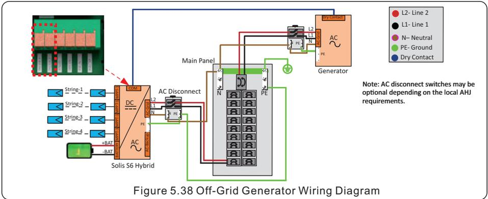
Figure 5.38 Off-Grid Generator Wiring Diagram
