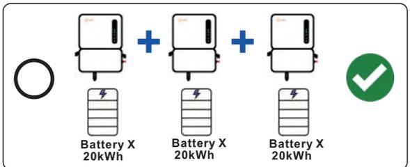
4. Do not install some inverters with batteries and some without batteries. Do not install different brand batteries on each inverter.
