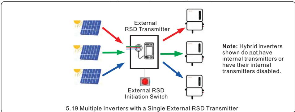
5.19 Multiple Inverters with a Single External RSD Transmitter
