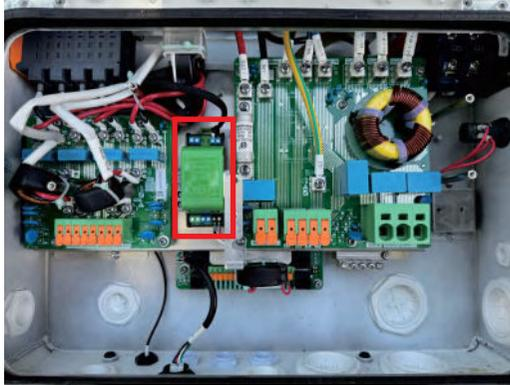
**Step 4:** Using a technician screwdriver, loosen the two terminals boxed in red. These are for the core that induces the PLC signal. Remove the two wires from the terminals.
