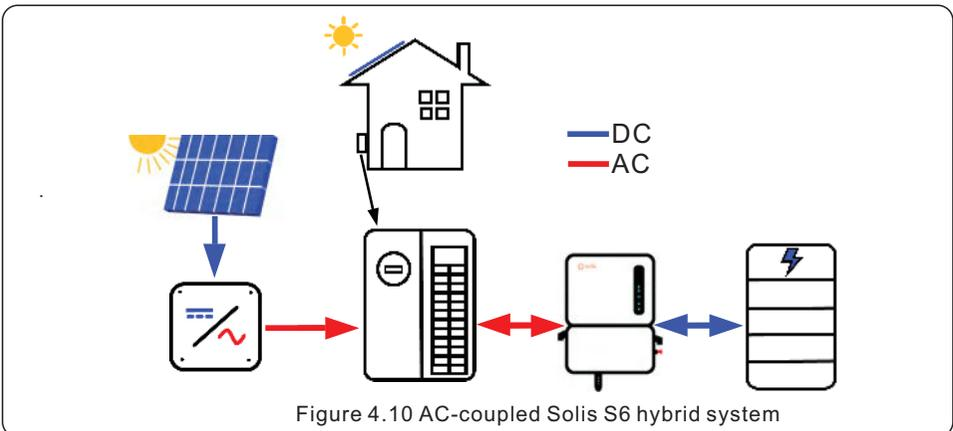
Figure 4.10 AC-coupled Solis S6 hybrid system
