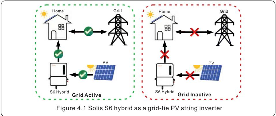
Figure 4.1 Solis S6 hybrid as a grid-tie PV string inverter
