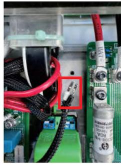
**Step 5:** Use electrical tape to cover the ends of the two core wires. Ensure the taped off wires are kept out of the way. Replace the metal cover plate with all five T20 fasteners.
