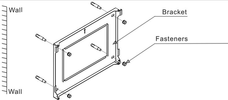
Figure 5.10 Fix the bracket to the wall
