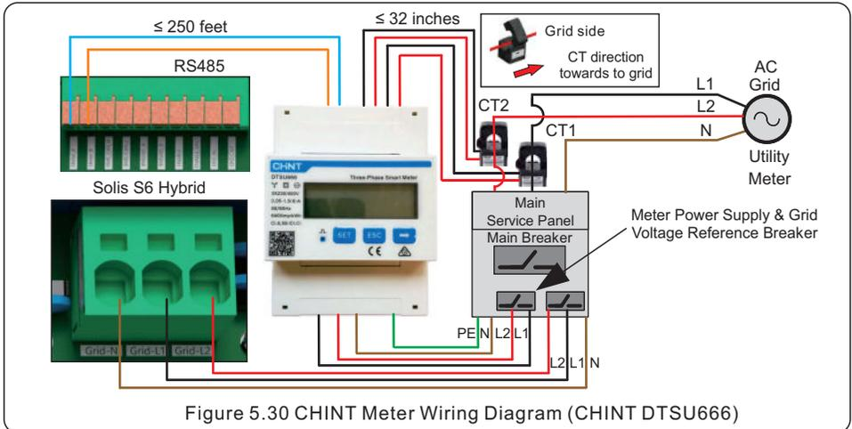
Figure 5.30 CHINT Meter Wiring Diagram (CHINT DTSU666)
