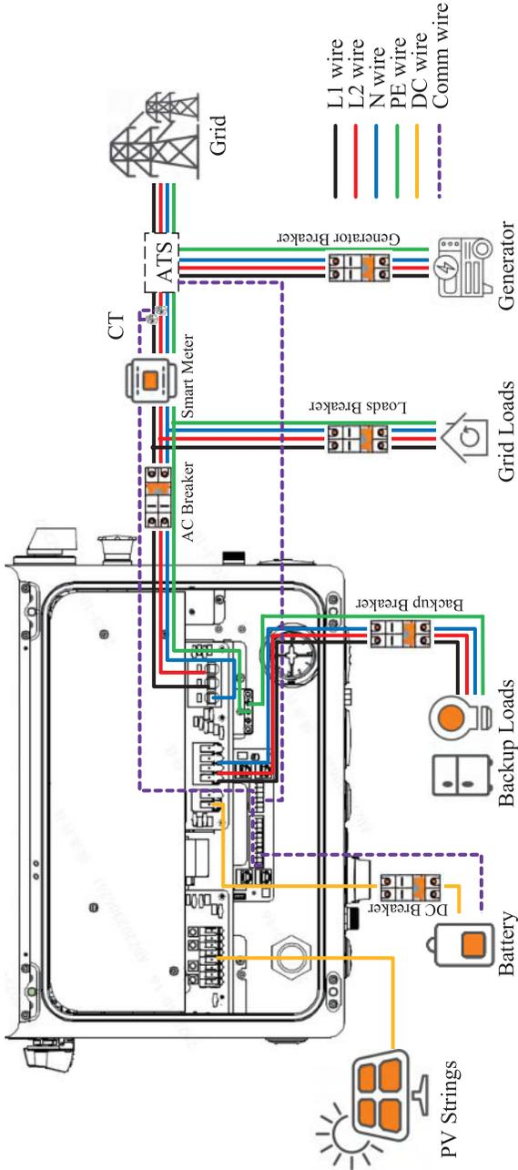
Figure 5.13 System wiring diagram with Generator and ATS
